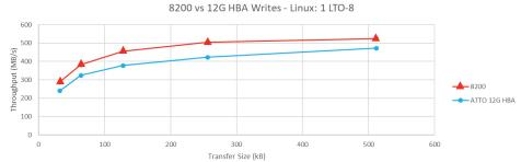
XstreamCORE ET 8200 writes are up to 20% higher over Ethernet than connecting directly to a SAS tape drive with a SAS HBA
