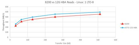
XstreamCORE ET 8200 reads are similar in performance experienced over Ethernet when SAS tape drives are connected to SAS HBAs
