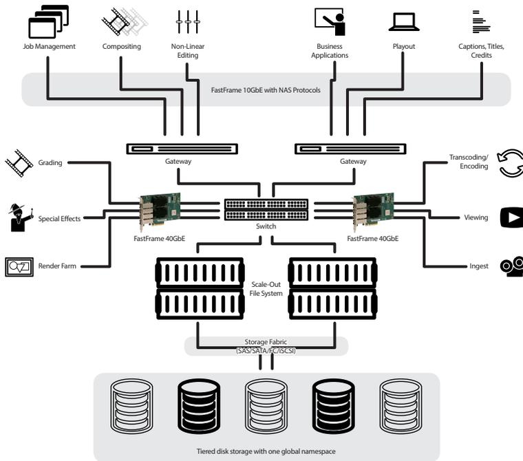
*ATTO 10GbE and 40GbE FastFrame NICs in a demanding 4k video environment utilizing NAS storage. This scale-out file system allows shared RDMA access to media storage, with support for one 4K/24fps stream for each workstation using RDMA. Areas in the workflow that don't require real-time uncompressed streaming utilize the gateway to access media files.*
