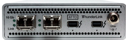
Dual 10GbE (SFP+ LC Optical) ports
