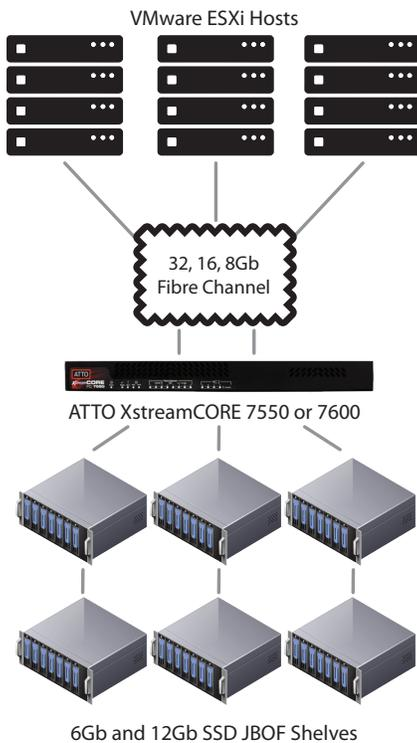
XstreamCORE connects up to 10 shelves of flash SSDs to a Fibre Channel fabric and then to up to 64 VMware ESXi hosts. This storage is then set up as remote flash for hosts or as SSD LUNs to scale up existing storage.
