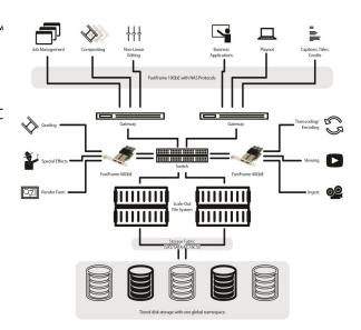
ATTO 10GbE and 40GbE FastFrame NICs in a demanding 4k video environment utilizing NAS storage. This scale-out file system allows shared RDMA access to media storage, with support for one 4K/24fps stream for each workstation using RDMA. Areas in the workflow that don't require real-time uncompressed streaming utilize the gateway to access media files.
