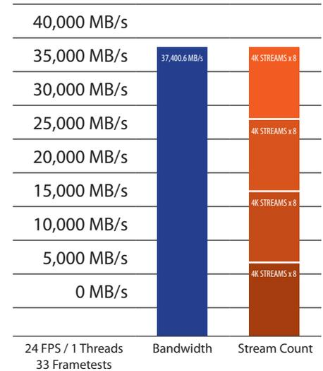
**RESULTS:** ATTO provides a consistent 32 streams of 4k with zero dropped frames. This results in a consistent 8 streams of 4k per client.
