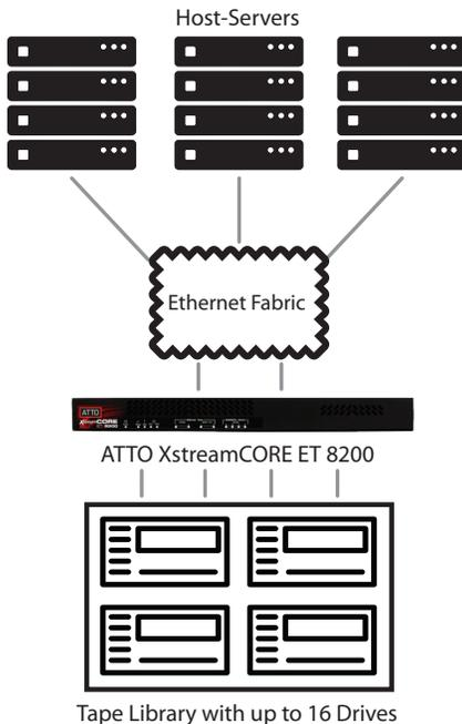
XstreamCORE connects up to 16 SAS tape drives to an Ethernet fabric using iSCSI over TCP/IP, iSCSI over RDMA (iSER) or Fibre Channel. This allows organizations to remotely locate tape devices while benefiting from lower cost SAS connected tape drives and libraries.
