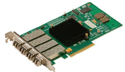
**Fibre Channel Host Bus Adapter
