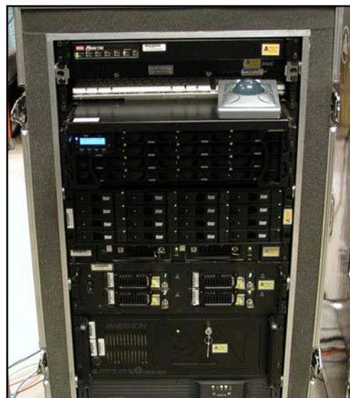
Advanced Audio put together a configuration that could be adapted to the changing needs of their clients. Featuring the ATTO iPBridge 2700 and ATTO's Xtend SAN iSCSI initiator, clients could connect their Macintosh via the Ethernet port directly into 3 Terabytes of online Fibre Channel RAID storage, or use 2 Gigabytes of Fibre Channel via the ATTO Celerity FC-42ES Host Adapter.
