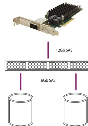
12Gb SAS/SATA, each link is capable of 1200 MB/s. With the exception of solid state drives, storage devices are not capable of saturating the link. With End Device Frame Buffering, more drives can work in parallel, increasing the overall performance of the system.
