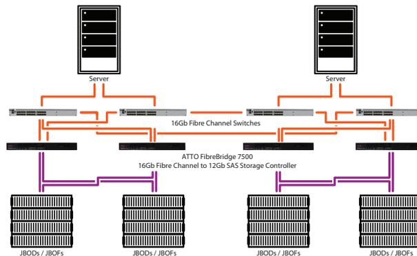
Highly redundant stretch cluster using multiple ATTO FibreBridge® 6500 or XstreamCORE™ FC 7500 storage controllers
