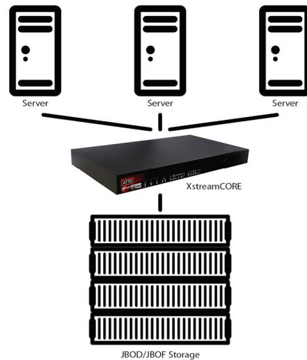
*XstreamCORE intelligent Bridges allows multiple servers running software defined storage to share off the shelf storage at high speed while adding features that accelerate and offload data transfers from host servers*
