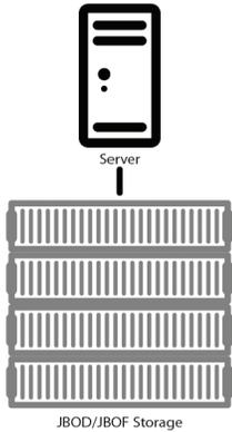
*Software defined storage architectures provide services and features at the server level. This allows one place to maintain feature licensing while using lower cost storage to architect a data center*
