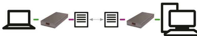
Fig. 2 - Media files are transferred from a laptop to a RAID-protected portable disk system. That same disk system can then be connected to a workstation for immediate content access.
