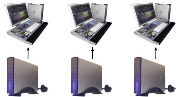
Direct Attached Storage
