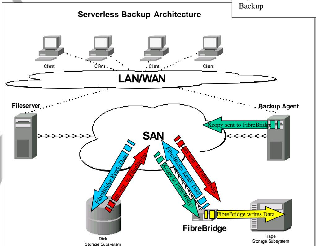
In this model, the server is just sending control data to the FibreBridge, using very little server resources
