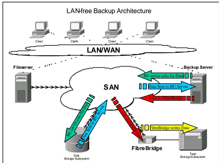
While the backup server still controls the data flow in a LAN-free architecture, the data path no longer goes through the LAN/WAN. The backup server reads the data from the disk storage subsystem. It then processes the data and Writes it to the tape storage subsystem. Because Fibre Channel protocol does not have packet collisions, the achievable data rates
