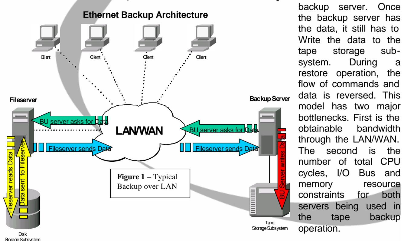
backup server. Once the backup server has the data, it still has to Write the data to the tape storage subsystem. During a restore operation, the flow of commands and data is reversed. This model has two major bottlenecks. First is the obtainable bandwidth through the LAN/WAN. The second is the number of total CPU cycles, I/O Bus and memory resource constraints for both servers being used in the tape backup operation.
