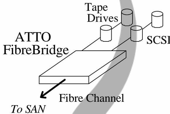
The ATTO FibreBridge™ not only converts the Fibre Channel protocol into SCSI, but also adds value to the SAN because it is an intelligent storage-management device. *intelligent Bridging Architecture* is the technology applied to move data efficiently and safely and is a collection of knowledge ATTO Technology has developed over the last 14 years.
