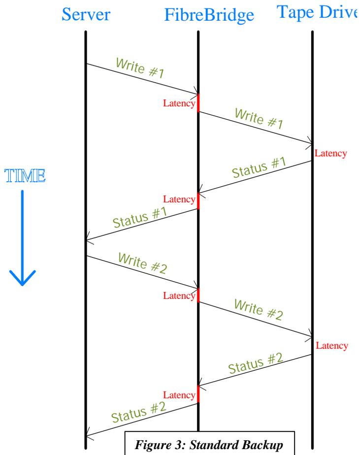
Figure 3 shows the flow of data during a backup as it passes from the server through a bridge, to a tape drive. A Write command must complete and the drive must respond with status before the next Write can begin. There is latency associated with the bridge as the command is processed as well as a time delay to actually write the data to the medium. The inherent sequential nature of tape drives together with a bridge reduces the overall bandwidth available to the backup process.
