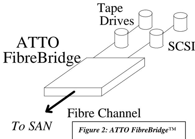
The alternative to native Fibre Channel tape libraries is to use SCSI tape drives and robot controllers with a Fibre Channel to SCSI bridge in front of it (see Figure 2). As Storage Area Networks emerge as the leading method to transition from server-based to storage-based architectures, companies need to focus on a total
