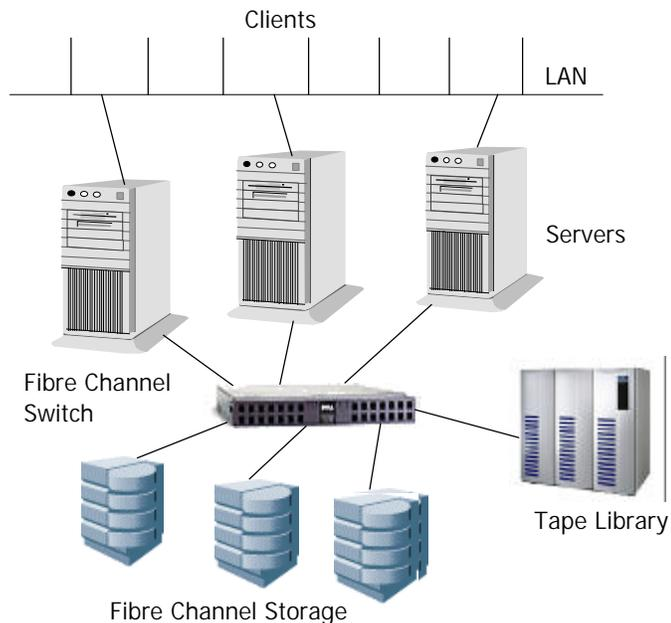
*Figure 1: Fibre Channel SAN*
