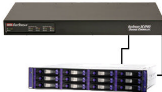
Exhibit 2 FastStream SC 5300 in split bus attached to a MediaDock II
