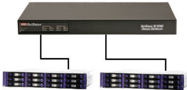
Exhibit 2 FastStream SC 5300 in split bus attached to a MediaDock II
