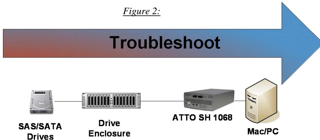
You begin with the device(s) connected to the ThunderLink SH 1068 first and work your way out to the host.
