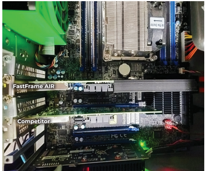
ATTO FastFrame AIR pictured installed in a workstation PCIe slot above a competing NIC. With the AIR baffling technology the FastFrame AIR NIC is half-height, 3/4 length, fitting inside most workstation and server chassis.
