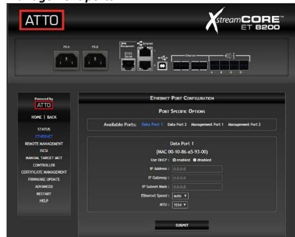
If you have completed configuration operations and have clicked **Submit** on the page you are viewing, go to the **Restart** page and restart the XstreamCORE to save the settings. Some settings may not take effect until the controller is restarted.
