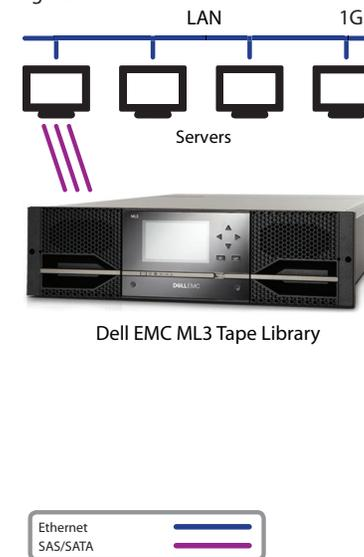
Figure 1: SAS tape libraries have distance limitations and connect on a one to one basis. Connectivity is typically done over a LAN connection with the server being the bottleneck and a point of failure if the server goes down.
